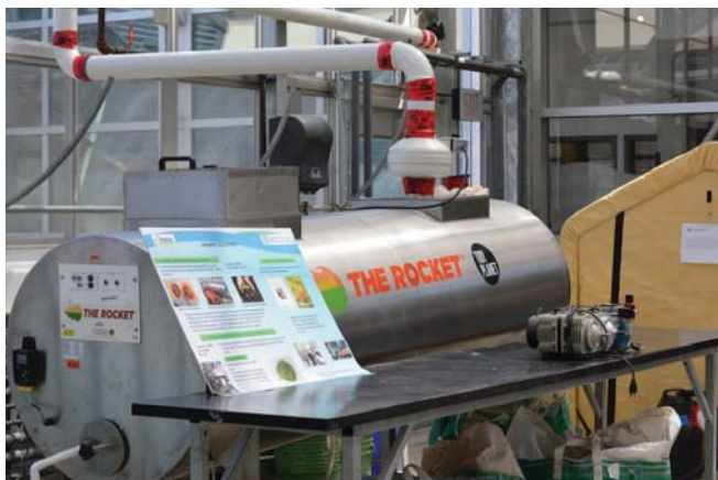
At Fleming, Applied Research has tested various configurations for The Rocket, a compost accelerator produced by MASS Environmental Services Inc. of Lakefield, ON.
